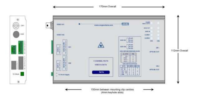
The **AMG5713A9-DIN** is a DIN Rail mountable standalone one channel video transmit unit designed to transmit 1 video signal and transmit & receive 1 data signal, 1 Bi-directional alarm and 1 Bi-directional audio channel over one Singlemode optical fibre.
